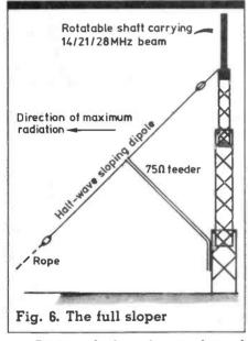
Best results have been achieved by using a slope angle of about 45° with the bottom end pulled out in the direction to be favoured. The metal tower tends to act as a reflector reinforcing vertically polarised radiation in the plane of the tower and dipole as shown in the diagram. A horizontally polarised component exists which is beneficial should short skip contacts be desired but, of course, gives rise to more By Sant Kharbanda C.Eng, FIERE, FSCTE, G2PU
