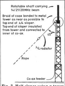
Fig. 7. Half sloper using a tower for support
