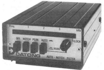
The value for money, stand alone automatic notch filter that doubles as a CW filter. Model ANF is small in size but neat in looks and big in performance. Simply connect model ANF in series with the loudspeaker lead of your receiver and from then on heterodynes, whistles and other steady tones that often make listening on the crowded amateur and short wave bands hard work will vanish automatically, as model ANF notches them out.
