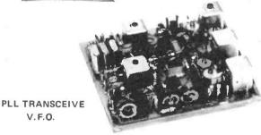
Converts any surplus radio telephone into a continuously variable F.M. transceiver. Microphone is connected to unit and a stable 2 metre F.M. signal is available for driving the amplifier stages. On receive the unit produces a local
