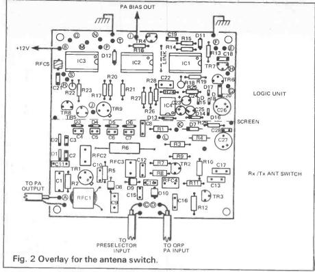
carriers created in the device provide an almost 'metallic' contact from collector to emitter. The alternative would have been to use a high voltage PIN diode at a cost of some several pounds. As it is, the BF259 does the job equally well and only costs a few pence.
