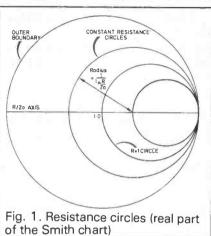
Chart is another tool, and the purpose of this article is to help you to find ways of using this tool, in the first case to help you to roll your own power amplifiers, and secondly, using the outer scales, to design an aerial. With this as a basis, you can follow by teaching yourself the other uses.
