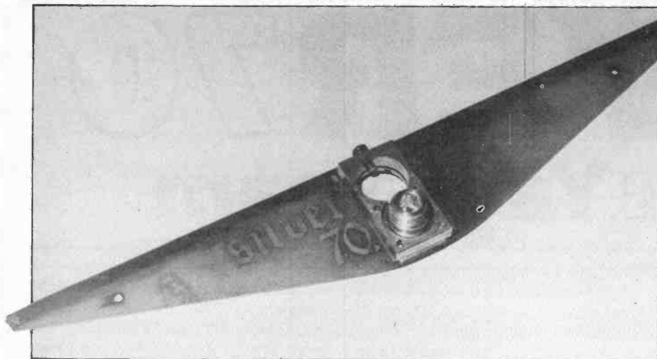
Driven element with 'N' type connection
