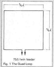
stacking distance between the upper and lower dipole 'halves'. A realistic figure for the gain dBd of the aerial (i.e. with reference to a single dipole) is in the range 1-2dB. The quadloop, however, unlike the half-wave dipole, appears not to be so fussy about its height above ground and, as I shall explain later, the effective gain is thus somewhat greater. 7MHz that had been missed by the club in its field day entries of previous years.
