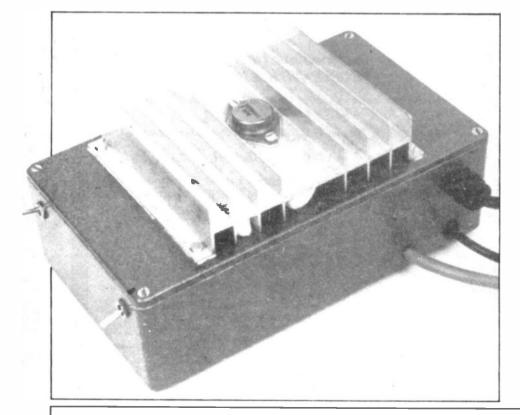
The operating power supply is built around IC1, an 78HG type regulator. The output voltage of this is set by R3 and R4, according to the formula.
