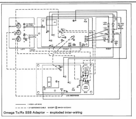
55mA, with point P at about 12V. With no output from the speaker, talk into the microphone and adjust RV4 (VOX gain) until point P reliably switches low as soon as you speak. The current should rise by about 10mA.
