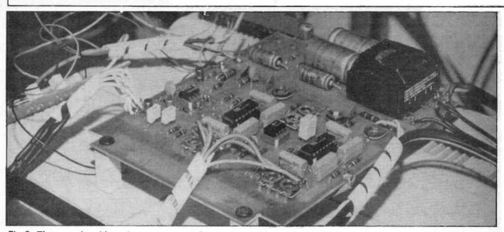
Fig.3. The completed board on test - not the neatest of assemblies, but it worked!
