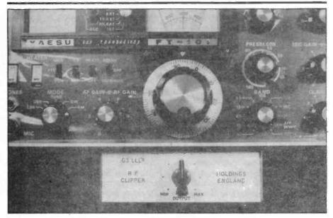
the case of the G3LLL Clipper, which is only made for the FT101, input and output connections are made by plugging the unit into the VFO socket, after attaching 3 jumper leads to spare pins.
