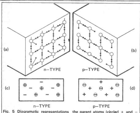
Fig. 5 Diagramatic representations of the front plates of n-type and p-type before fusing together (a and b), and in simplified form showing just
