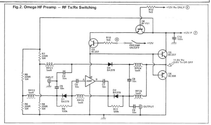
inhibit parasitics associated with the transformer leakage inductances. The amplifier provides a flat gain of 15dB across the HF spectrum when correctly terminated on both input and output into 50 ohms. It has an output capability of + 15dBm (about 30mW.
