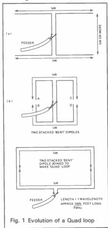
Fig. 1B as points A & B and also  $\overline{\mathbb{C}}$  & D are in phase and have the same voltage on them so that they do not need insulating from each other. Once they are connected together, as in Fig. 1C, the top feed point is no longer needed as energising the lower ''dipole' also energises the upper one, and this how the classic quad loop is formed.
