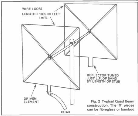
The exact shape of a Quad element does not seem to matter much, provided that the formula length of wire in feet equals 1005/F(MHz) is not taken too literally, and the possibility of adjustment of a few per cent is allowed for either way. Squares, diamonds, circles and triangles all seem to give good results, but, of late, the latter, which for some reason has been re-christened the delta loop, has become very popular.
