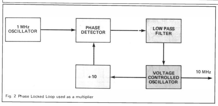
ed. As phase is the differential of frequency with respect to time this means that when the phase difference between the two signals is constant then the two frequencies are exactly the same.
