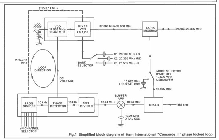
c=10.695 MHz (1st IF) d=37.660 to 39,000 MHz (high LO/VCO output) e=2.55 to 2.11 MHz (VCO output to Prog Div) f=26.695 to 28.305 MHz (Tx/Rx freq)
