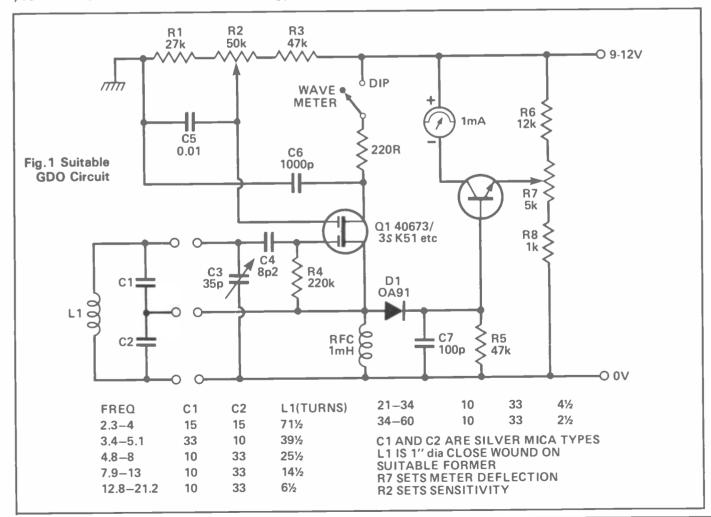
A circuit is given for your interest (Fig.1) — it does work! The device may be simply calibrated by listening for the output on a suitable receiver and calibrating from the receiver dial or digital readout.
