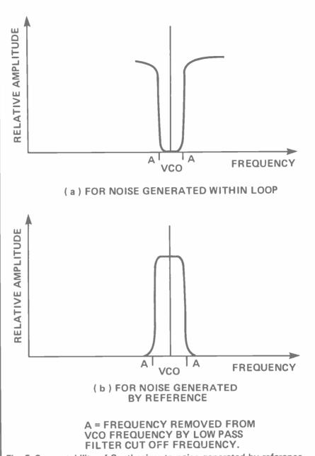
Fig. 5 Susceptability of Synthesiser to noise generated by reference and loop.
