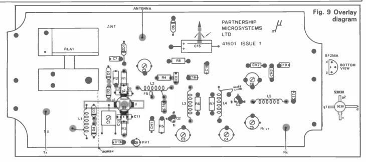
fit inductors L1-L5 and the respective taps, the axes of L3 and L4 must be parallel and 15mm apart. Use a minimum of heat consistent with good joints.
