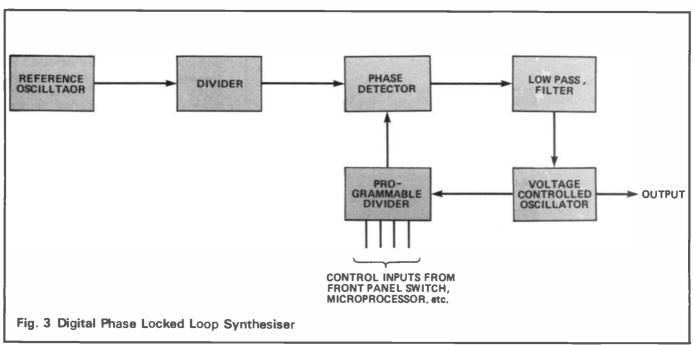
channel spacing, and the programmable divider will have to give division between 5800 and 5840.
