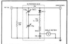
Fig. 14 Circuit of 27 ohm series resistor
