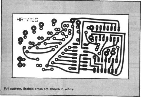
Fig. 4. shows the completed PCB layout which was sufficiently small for placing inside the converted rig. After constructing the unit, the following conversions will need be made to the display area of the rig.
