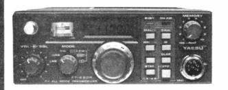
FT290R "MULTIMODE PORTABLE" Multimode 2M Transceiver Dual VFOs Microprocessor Control Selectable Synthesiser Steps Large LCD Display Ten Memory Channels '+' & '-' Repeater Function Nicads for Portable Available 2.5W / 0.5W RF Output 58(H) × 150(W) × 195(D) mm
