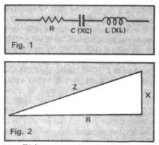
This can be reduced to  $Z = \sqrt{R^2 + X^2}$ . If we think back to our basic tuned circuit theory, X = X L-XC. At resonance Z = R, the resistance of the tuned circuit, because XL. the inductive reactance of the tuned circuit, is equalled and cancelled out by XC, the capacitive reactance of the circuit. **\*** (By the way, reactance can be defined as the term given to the opposition to AC current flow in a
