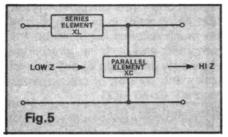
The simple L network shown nearby in Fig.5 will transform a low impedance to a high impedance if connected as shown. By reversing the input and output a high impedance will finish as a low impedance. The observant reader will spot something straight away (See Fig.6 for an extra hint).
