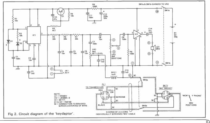
keyed audio tone through when switched to MCW. Switch SW2B provides PTT (push-to-talk) override. In MCW mode, normal PTT facility, available at the microphone, is overridden, the transceiver being put into the transmit mode. With SW2B in PHONE position, normal PTT is restored.
