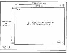
cremented one space, if the new cursor position is greater than the old then the cycle is repeated. When the last cursor position on the screen is reached however, the next increment will result in the wrap-around effect, HO will be 0 and CO will be 39 - so as soon as HO becomes less than the value of CO, the edge of the screen has been reached and the total number of columns is the same as the value held by CO.
