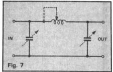
The idea is to transform the typically high output impedance of the valve down to about 25 ohms and then step it up to between 25 and 500 by making the capacitors variable and the coil tapped. The centre transformation point varies along the coil with frequency and finds its own balance point. The value it transforms down to in the centre of the coil is about 25 ohms. Look further into this arrangement and converting it to a real life situation
