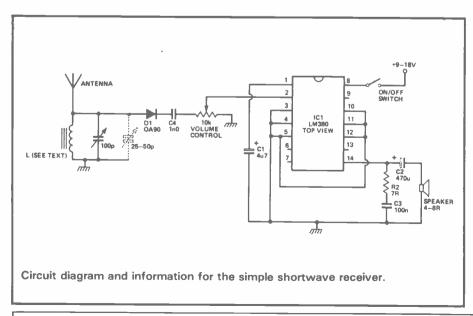
stator lug of the 100pF capacitor, C, and the other end to the frame (rotor). Solder D to one of the stator lugs using a heat sink (ie grip the end of the diode being soldered with a pair of long nosed pliers). Should the tuning of the receiver prove to be too sharp, a 20 or 25pF variable capacitor may be connected in parallel with VC1 (see Fig.1) to act as a bandspread capacitor (ie for fine tuning).
