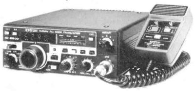
290D is the state of the art 2 meter mobile, it has 5 memones and VFO's to store your favourite repeaters and a priority channel to check your most important frequency automatically. Programmable offsets are included for odd repeater splits, tuning is 5KHz or 1KHz.
