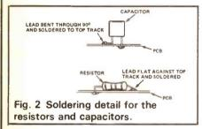
all RF circuits it is important to keep all component leads as short as possible; lay resistors directly on the board, keep capacitor leads to a minimum and mount transistors Q2 and Q3 with lead lengths 3-4 mm.
