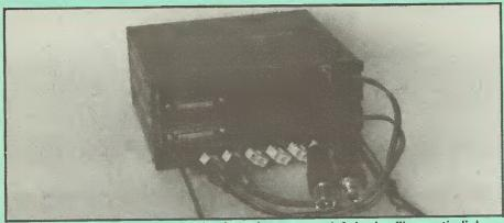
Rear interconnections, the thin lead on the extreme left is the fibre optic link
