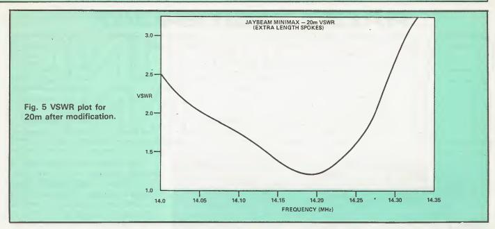
duction of the LF end VSWR. This does show that the mounting location certainly has an effect on the beam.
