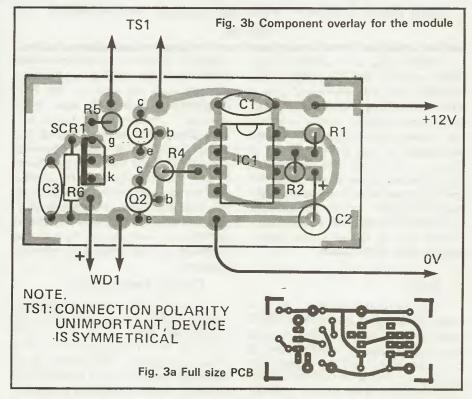
The sensor TS1 is in fact a solid state thermal switch which is normally about 100k resistive, but rapidly drops to 100R or so when it reaches 75°C — when it cools the resistance rises again to the 100k value. Whilst NPN and PNP silicon transistors run quite happily at 75°C, the thermal switch can be mounted
