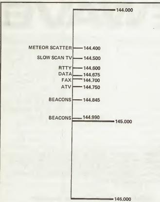
Fig. 1 The chart shows the amount of frequency area below 145MHz available for FM communication. FM should never be used above 144.845MHz as it may blot out weak signals from distant beacons. If used below 144.5MHz this should be done circumspectly because (a) the 'all mode' section stops here and (b) SSB may be present.
