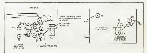
Fig 1. Construction details of the RF front-end (capacitor marked C is 10n to 100n bypass capacitor).
