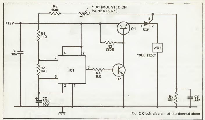
to provide an unequal mark-to-space square wave output at pin 3. The frequency in this instance is approximately 5Hz.
