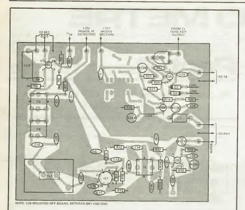
Fig 2. Layout for the main PCB and foil pattern. The capacitors marked simply C are decoupling capacitors, with values of 10n to 100n, depending on what you have to hand.
