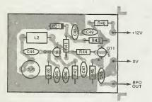
Fig 4. Layout of the BFO board.
