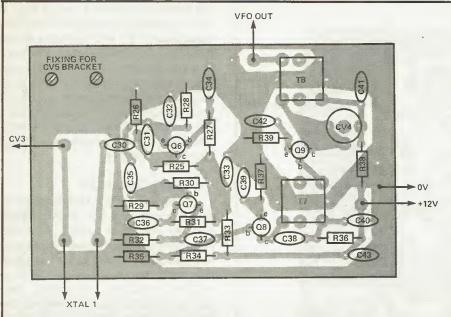
Fig 3. Layout of the VFO board.
