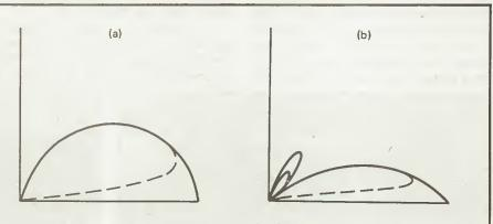
Fig. 1 Vertical polar diagram of (a) a vertical quarter wave and (b) a vertical half wave aerial with its centre a half wavelength high. The solid line indicates the pattern which would be obtained over perfectly conducting ground — the dotted lines show the pattern over imperfectly conducting ground.
