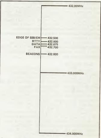
Fig. 2 In the 'all modes' section of 70cm no less than 300kHz are available for FM QSY. Never QSY into the beacon segment above 432.8MHz and avoid the three specialist spot frequencies shown.
