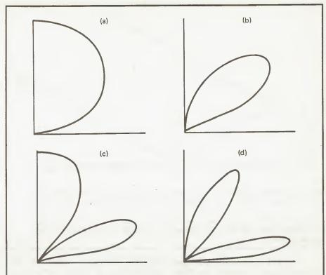
Fig. 2 Vertical polar diagrams for a horizontal half wave aerial when at a height of (a)  $\frac{1}{4}$ , (b)  $\frac{1}{2}$ , (c)  $\frac{3}{4}$ , and (d) one wavelength.
