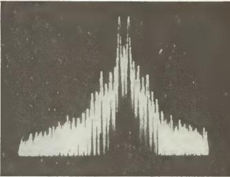
35W PEP input signal (left) and resulting amplifier output (right) of 400W PEP on 20m
