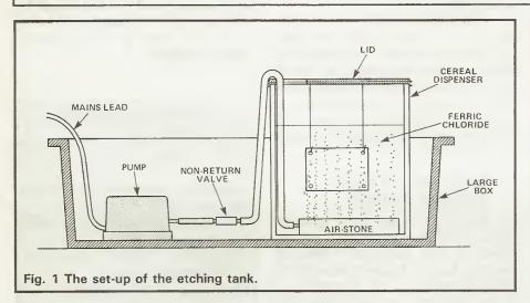
Many accessories are now available for the production of printed circuit boards at home. Marking the tracking pattern on to the unetched copper-clad board can be achieved by using an etch resist pen, etch progress has some drawbacks: it requires manual agitation to ensure quick, even etching and the solution can easily be spilt or splashed.
