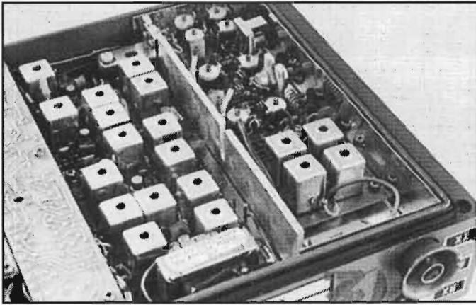
Use a suitable non-metallic trimming tool for aligning the fragile cores
