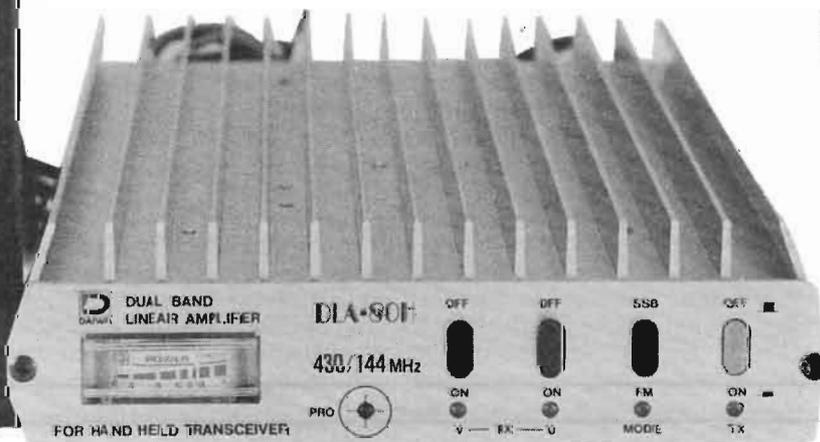
gain a greater benefit from the very low noise figure of the GAsFET preamps. Occasionally I found that when I transmitted on the lower part of 2m I had some receiver desensitisation on 70cm when listening to a weak signal with the preamp switched in, this was probably caused at the receiver end because of third harmonic noise sidebands. In the end I normally ran with the preamps switched out, this always superb twin-band operation.
