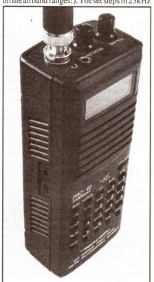
steps on the 118-136.975MHz VHF airband range, 5kHz increments on 68-88MHz, 137-174MHz and 220-225MHz, and 12.5kHz increments on the remaining frequency ranges.
