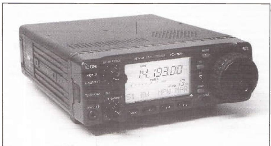
graphically reduces when you switch this in. A switchable preamp, attenuator, and an RF gain control (which sometimes isn't found on such small sets!) plus a pulse-type noise blanker add to the QRM-fighting measures. Besides the 2.3kHz, 6kHz (AM) and 8/15kHz (FM) filter bandwidths fitted as standard, optional filters of 1.9kHz and 2.8kHz are available for SSB, RTTY and CW, and 250Hz and 500Hz for CW/RTTY.
