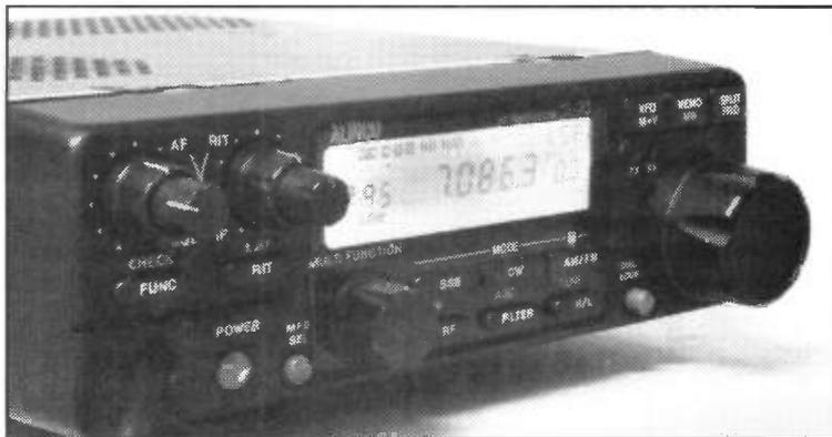
I found the set was quite easy to use on the move, although I had to be careful in using the front panel VFO knob in a moving car - I often 'overshot' on tuning. Instead, using the transceiver's 'set' mode, I set the mic up/down buttons to tune and scan in 100Hz steps, thus making mobile tuning a piece of cake. The set was small enough to fit below my dashboard, and after
