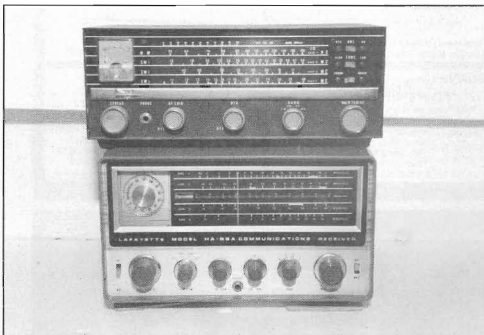
Typical sets that could be used to experiment on without great expense. The top set is the Realistic short wave set, 4 valves, with a Lafayette HA-63A below, this is a 7 valve set. Both have bandsread, and S meter and a BFO function.
