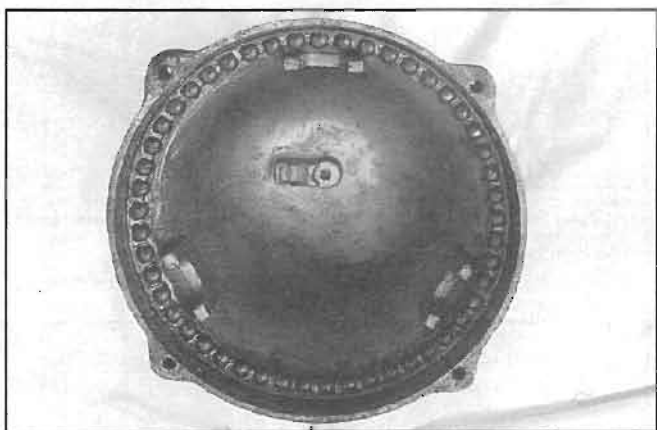
Looking up into the bell housing, you can see the recess for the indicator pot. The three lugs on the rim are the locating slots for the lower power unit.
