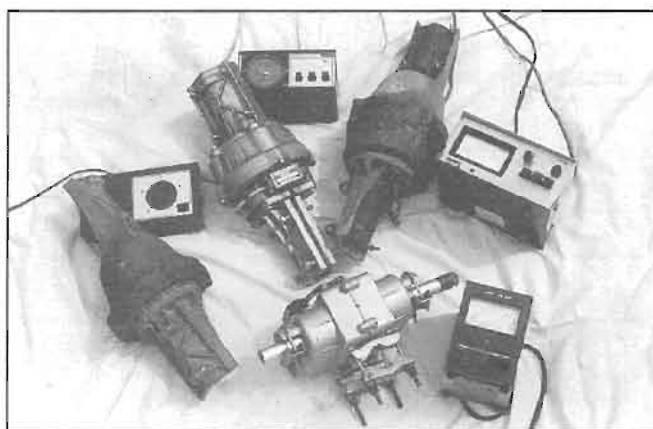
A selection of rotators, shown from left to right.. AR30 (lightweight use, i.e. VHF/UHF array). Daiwa heavy duty rotator (suitable for large VHF arrays or for HF tribander types). CDE heavy duty rotator (as Daiwa). KR500 elevating rotator (ideal for satellite arrays, relatively light weight only).
