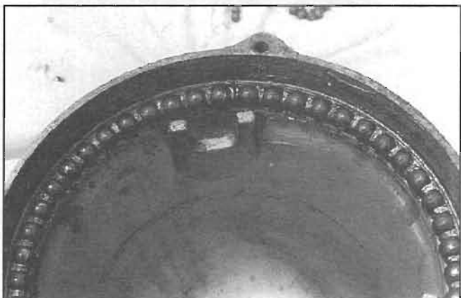
Clear view of the locating slot and ball bearings. In cheaper versions of this same rotator only a few bearings will be found.
