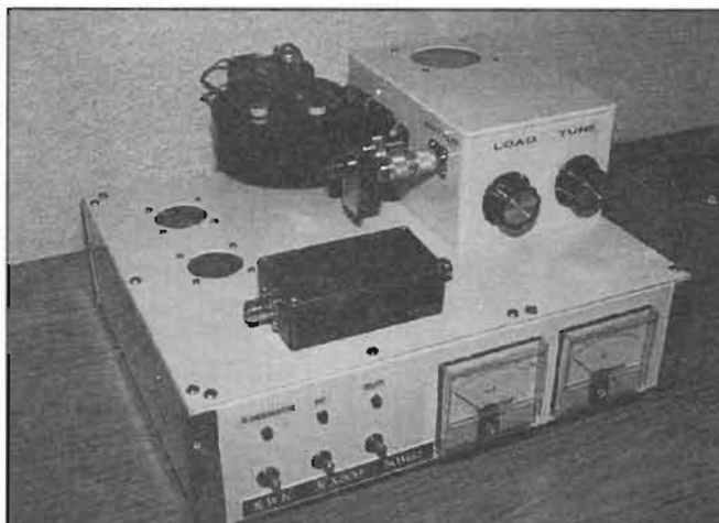
50MHz legal limit amplifier, including power supply and 500W low pass filter, there's a full construction article on the way this winter for Ham Radio Today!
