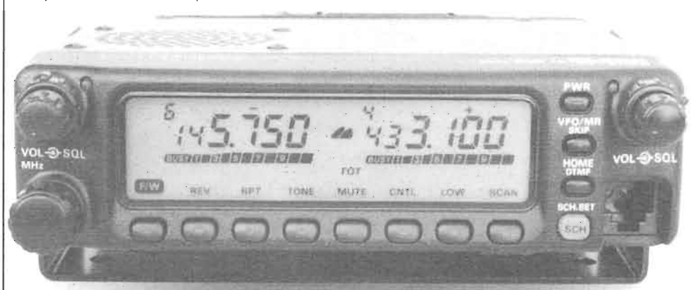
A tiny high-powered mobile. The front panel has independent volume and squelch controls for each band
