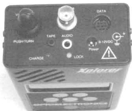
The Xplorer has an audio output / headphone jack plus a 'tape control' jack to allow for automatic recording.
