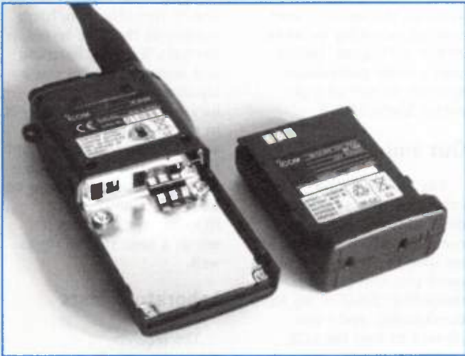
A clip-on 7.2V nicad is supplied which gives 3.5W transmit power output
