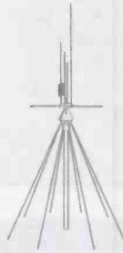
**Skyscan DX-V1300 base discone** – Most discones only have horizontal elements and this is the reason that they are not ideal for use with a scanner. Most of the transmissions that you are likely to receive on your scanner are transmitted from vertically mounted antennas. The DX-V1300 has both vertical and horizontal elements for maximum reception. Constructed from best quality stainless steel and aluminium and comes complete with mounting pole. **£49.95** + £3 P&P.
