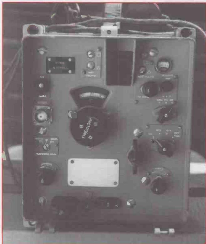
The R-326 receiver. The window top centre lights up to display the frequency scale.
