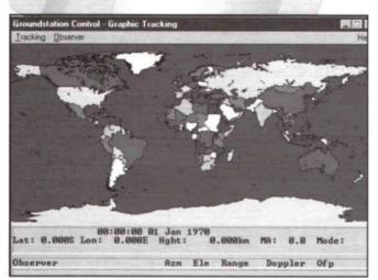
WiSP gives you total station control, including showing you when the satellites are in range and even controlling your station automatically
