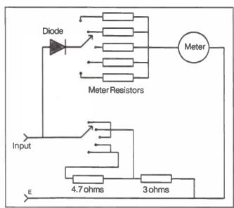
Fig.4. The complete circuit of the Audio Output Meter
