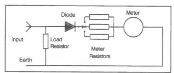
Fig. 2. Modification to basic power meter circuit for multiple ranges
