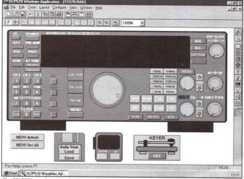
The TS-570D can be remotely computer controlled from your PC by using an RS-232 interface. For this, Kenwood can also usefully supply suitable custom-written software
