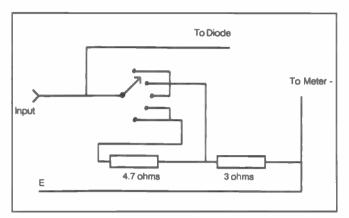
Fig. 3. Switching arrangements to permit both 3 and 8 ohm operation
