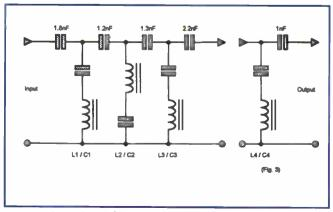
Broadcast band filter circuit, high pass above 2MHz
