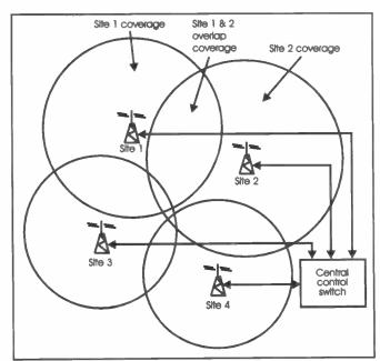
Quasi-synchronous operation gives wide coverage on a single VHF/UHF radio channel
