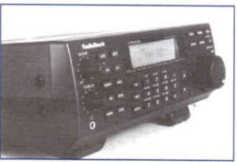
A rotary 'tuning' knob can be used for channel selection. A 3.5mm jack socket is provided on the front panel for headphone use, this can also be used for plugging in an amplified extension speaker
