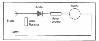
Fig. 1. The basic circuit of a simple power meter
