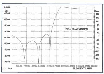
Fig.4. Final version for the 160m band
