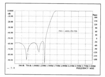
Fig. 1. ARRL 10 pole BC filter response chart
