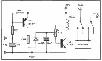
Lower the power on your transmitted signol with this simple relay changeover circuit
