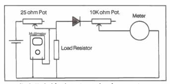
Fig.5. Method for determining value of meter resistors
