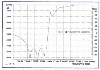
Fig.3. 13 pole filter version using a 2mH choke as the load
