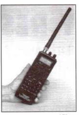
The receiver measures 171 x 62 x 40mm and weighs 229g, it fits comfortably in the hand
