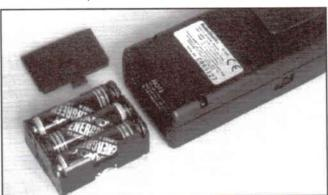
Six AA batteries are used for power, these fit into a battery pack which slides into the case
