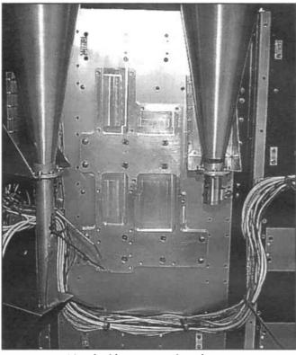
10GHz feed horns mounted on Phase 3D
