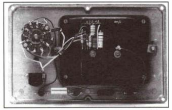
Internal view, the load resistors are below the meter and the dropper resistors are mounted on a piece of Veroboard attached to one meter terminal
