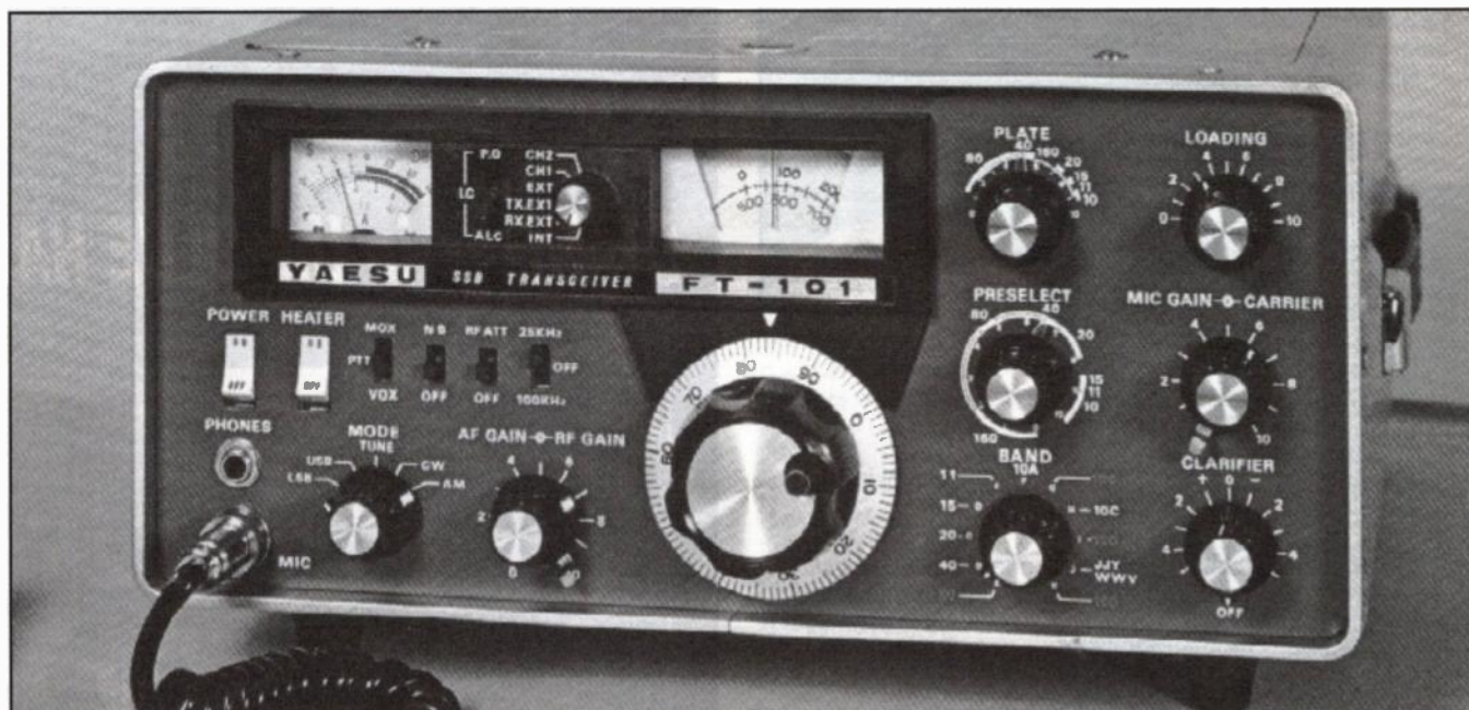
Clifford came with his FT101 with the complaint that it would not switch over to transmit quickly enough, and that sometimes the receiver took several seconds to recover after transmitting.
