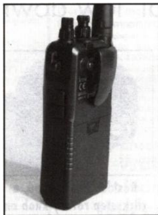
The IC-R10 measures 58mm wide x 130mm high x 31mm deep, and weighs 310g.
