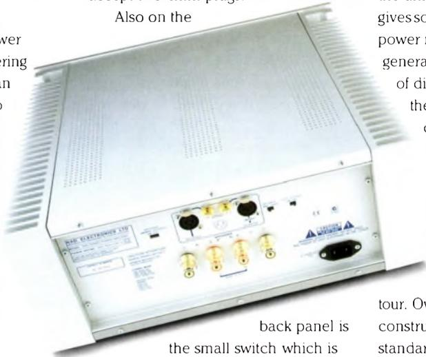
back panel is the small switch which is used to engage NAD's proprietary 'soft clip' technology. As its name suggests, the idea of this additional circuitry is to round off a square, i.e. clipped, waveform to minimise distortion produced by the amplifier as it runs out of steam – should that ever
