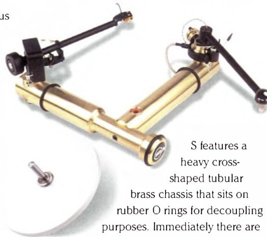
S features a heavy cross-shaped tubular brass chassis that sits on rubber O rings for decoupling purposes. Immediately there are cost savings; no plinth, no lid, not to mention much reduced assembly time.
