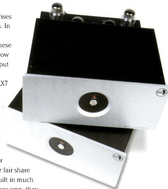
All the filament supplies are rectified and smoothed, including the power valves, which as far as I know is unique in a commercial design.
