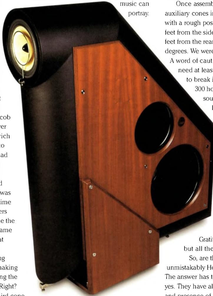
The famed 3kHz midrange honk of the Lowther is a narrow band distortion, and according to Jacob, is a result of the intermodulation between the whizzer and the cones in the driver. By interposing a third cone acting as a baffle, which does not touch the other two cones, you ameliorate the potential uplift so often heard with this driver. The cone is held in place by being fixed to a chrome ring,
