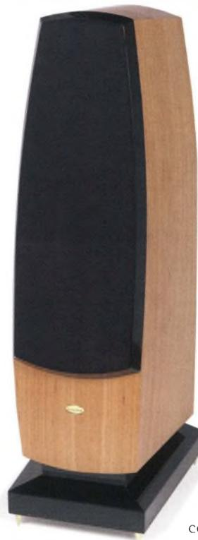
▶ same silky velour material as the very tactile grille cloth. The enclosure is damped and mass-loaded by lead sheeting, while the avoidance of parallel faces will serve to spread out the frequencies of the standing waves generated internally.
