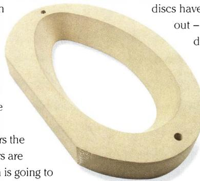
discs have an egg-shaped cut-out – an ideal shape for distributing standing waves and reflections, while also creating variable thickness walls. And the inside back edge of each disc has a 45 degree chamfer in order to deflect rear radiation from the driver downwards rather than back through the cone. Light damping around the middle of the tower helps absorb the vertical standing wave.
