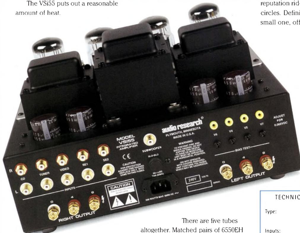
Obviously, the valves get fairly warm, but less predictably so too does the mains transformer and (to a much lesser degree) the two output transformers. With the latter, the rise in temperature is almost certainly down to heat conduction from the four output tubes and mains transformer. Certainly, after the amp's been on a couple of hours or more, the whole case warms up.
