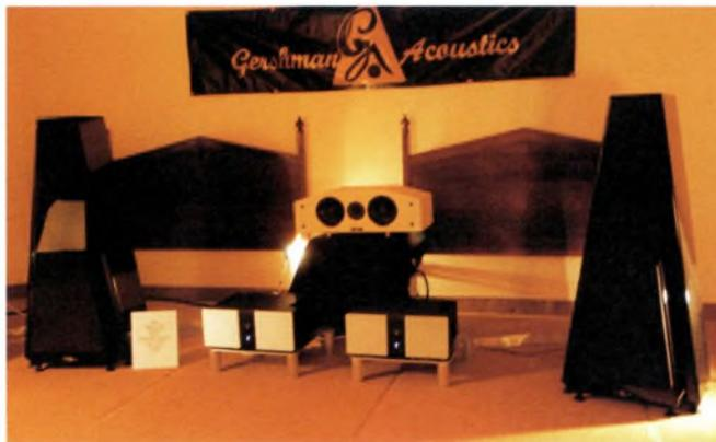
employing top-flight Scan drivers in a d'Appolito arrangement. The tapered, trapezoidal cabinets weigh around 75kgs each and feature external crossovers, loaded with such goodies as Hovland caps and Alpha-Core coils. The walls range between an inch and three-inches in thickness, with internal compartments further damped with a mix of lead-shot and sand, which
