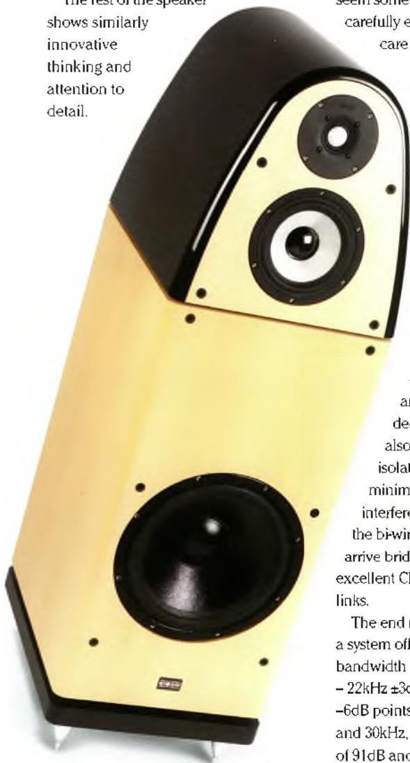
The one-piece head unit is a composite molding sandwiching a structural foam core, delivering low-mass and excellent self-damping. The resultant 15 litre enclosure exhibits very low stored energy and thus low levels of mechanical and intermodulation distortion, while the asymmetrical shape helps kill internal
