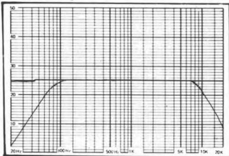
A typical pen chart of the tone controls with rumble filter.
