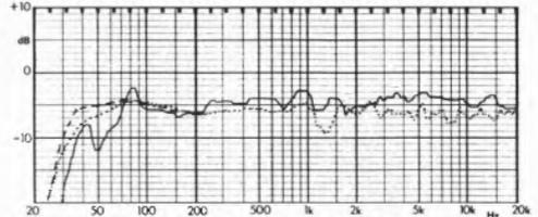
Axial sine wave reference response, 1m (0dB=90dB sensitivity; dashing corrects chamber anomalies.) (solid curves Mk I, dotted Mk II.)
