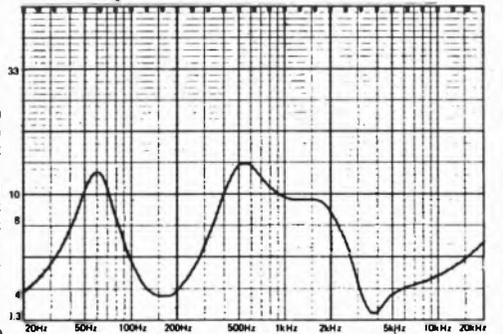
below: averaged frequency response at 2m (solid curve on axis, dotted curve 10<sup>0</sup> vertical, dashed curve 30<sup>0</sup> horizontal) vertical scale 1dB/div.
