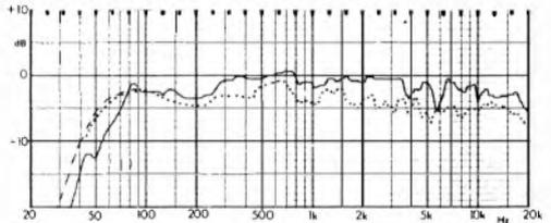
Axial sine wave reference response, 1m (0dB=90dB sensitivity; dashing corrects chamber anomalies.) (dotted second sample)
