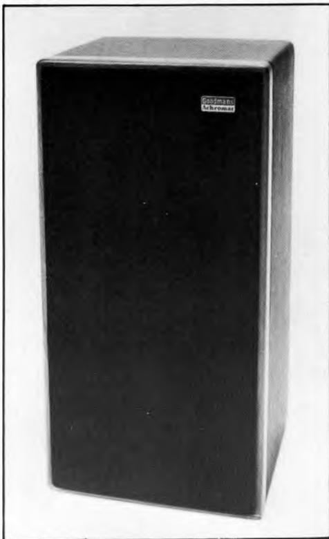
Representing the middle sized model in the new Achromat Series from Goodmans, the *Kappa* is a small 25 litre, two-way sealed box system some 54cm high. Of unusual styling, the cabinet is finished in a soft-touch, grained leather-look vinyl, with the front edge framed in a lighter hardwood nosing. Constructional quality is good and the cabinet is braced internally, with full bituminous panel damping as well as an acoustic foam lining and an acrylic wool filling.
