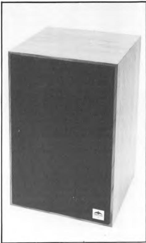
This 14 litre sealed-box system is only 36cm high — just about the smallest enclosure that could take a 200mm Dalesford bextrene cone mid/bass driver, and a KEF T27 tweeter. The crossover is a fairly simple 8-element type, built with fine, high power components.
