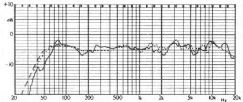
Axial sine wave reference response, 1m (0dB=90dB sensitivity; dashing corrects chamber anomalies.) (dotted curve 2nd sample)
