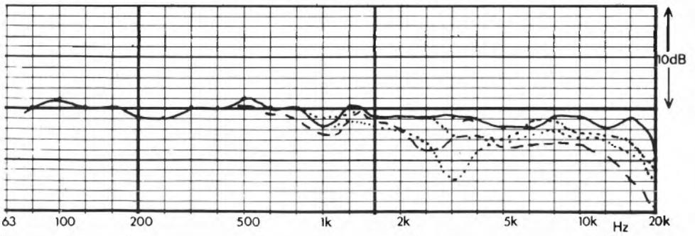
1-octave averaged frequency response. 2m solid axial; dotted 10 dB above and below; dashed 30 dB horizontal
