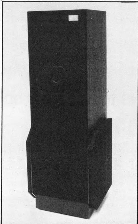
Similar to the larger AR9, the 90 makes a small concession in ultimate power handling and bass extension by allowing the use of two 250mm low frequency drivers per enclosure instead of the 300mm units used for the '9s. The remaining drivers are the same, namely a 200mm pulp cone midrange a 38mm soft dome lower treble, and a 19mm soft dome upper treble, arranged in a vertical-in-line format. An 'acoustic blanket' (a thick felt layer) surrounds the drivers.
