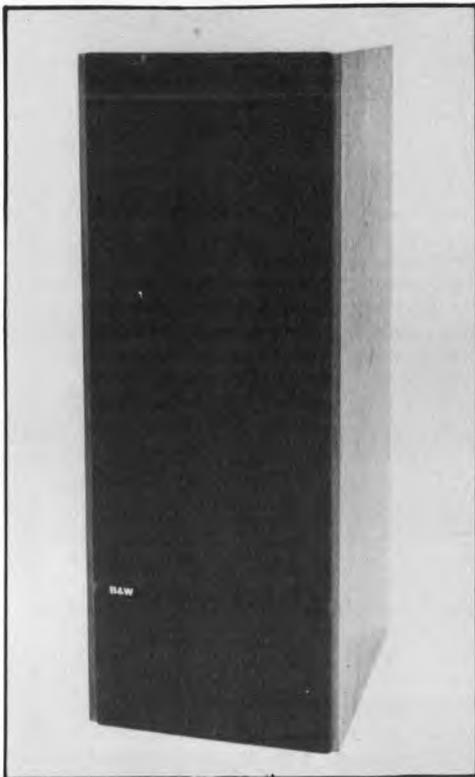
This tall, slim enclosure was accompanied by a steel pillar stand with a veneered base, and the whole may be bolted together for improved rigidity and stability. Carrying the legend of an earlier and long lived B&W system, this Mark II version in fact bears little resemblance to its predecessor.
