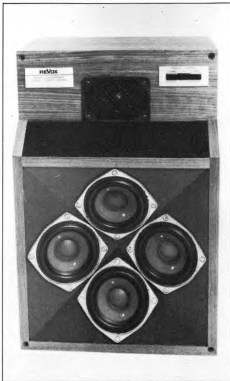
The *BX350* represents a new and serious entry into the loudspeaker market for Revox. A 'linear phase' system, the treble driver is set back on the stepped front baffle to bring it into time alignment with the bass-mid array, an open frame grille exploiting the gap to the upper cabinet step as a deliberate visual feature. Pushbuttons allow selection of treble output in 2dB steps, and as the system is quite compact, it is presumably primarily intended for shelf mounting.
