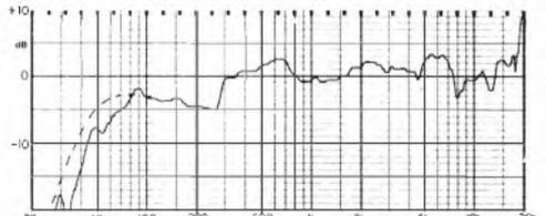
Axial sine wave reference response. 1m (0dB=90dB sensitivity; dashing corrects chamber anomalies.)
