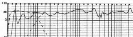
Solid: axial sine wave reference response with satellite; dashing shows chamber correction and crossover slopes.
