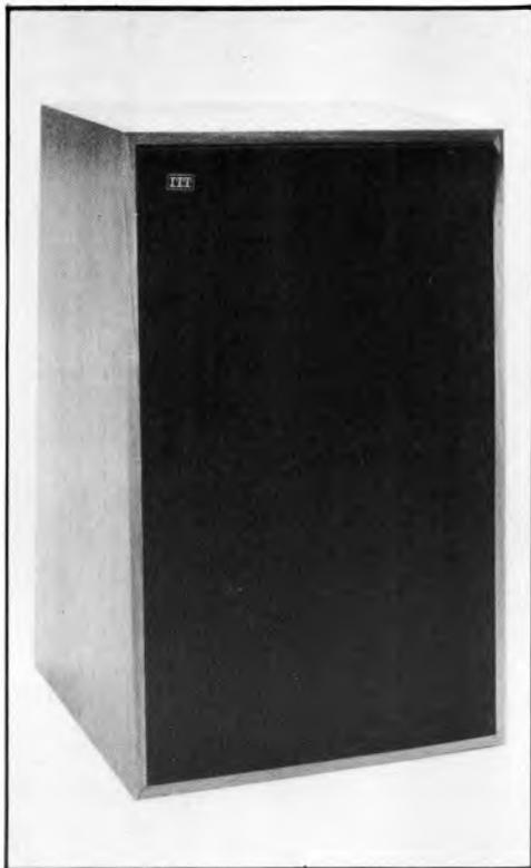
The 8072 is the median model in a range of UK designed speakers that incorporate Audax drive units. Having a fairly squat appearance, a two section tilted-back grille is employed, the upper section being detachable to reveal two controls for adjustment of lower and upper treble. These frequencies are handled respectively by 37mm and 25mm soft dome units mounted laterally adjacent on a diffraction-inducing recessed panel above the 200mm bass midrange driver.
