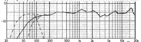
Solid: axial sine wave reference *JR150*, dashed shows subwoofer extension (corrected) and crossover slopes.
