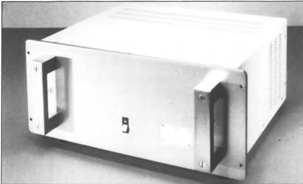
An American heavyweight built to the highest standards of finish and construction, the KSA50 is a very expensive power amplifier modestly rated at 17dBW (50W). Versions at 100W and 200W are also available, and with the exception of the power output, these are broadly similar in performance to the '50.
