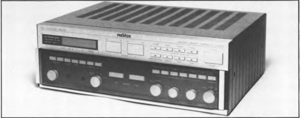
Part of a new range of high-quality electronics, the Revox *B251* is a generously-powered amplifier with a fully equipped front panel catering for almost every conceivable need of the technically-minded enthusiast. Not surprisingly perhaps, some of the numerous features are directed towards tape recording, such as the accurate peak-responding meters which can be directed to show gain, balance level and output power.
