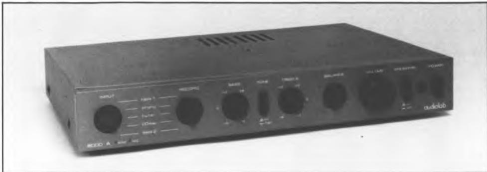
A brand new amplifier, the 8000A is intended to be one of a new range of electronics designed by two UK engineers with an established track record in this field. It is conservatively rated at 50W per channel.
