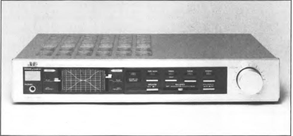
Rated at 38W per channel, the AK-22 is an inexpensive integrated model which sells for under £100. Finished in silver and blue, it has a low-profile format and facilities include connections for two sets of speakers, via clamp spring terminals. Inputs are provided for tape, video (aux), tuner and disc, while the slider-type bass and treble controls are supplemented by a loudness button. All input sockets are phonos.
