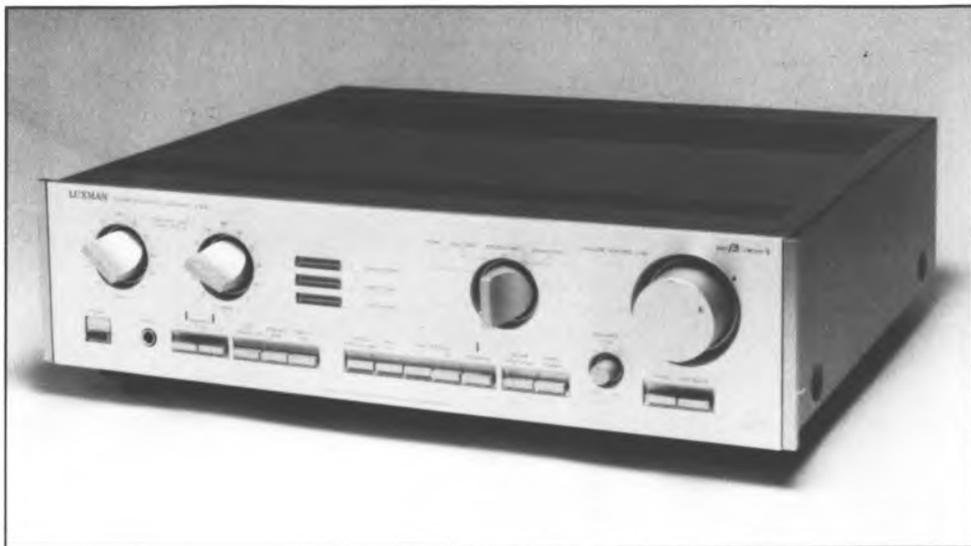
Well-presented and finished in the usual Lux manner, the L230 is a medium-priced integrated amplifier and comes with a comprehensive specification. Rated at 60W per channel (17.5dBW), it offers moving-coil and moving-magnet disc inputs plus tuner and aux/CD and facilities for two tape decks.
