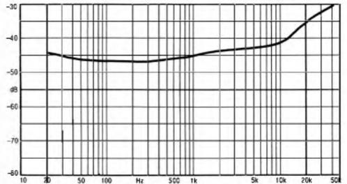
Disc input: stereo separation
