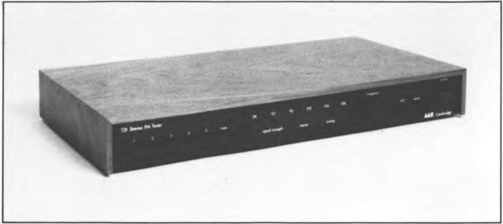
An established British tuner which matches the A&R A60 integrated amplifier, the T21 is a slimline model with a walnut veneered surround sleeve. An analogue-tuned design, it has a varicap front end, and the coarse tuning dial is composed of a number of red LEDs. Up to five stations may be pre-set via a row of knobs on the rear panel, with the manual tuning set to a sixth station or used for further selection. A mono switch and afc button are both fitted.
