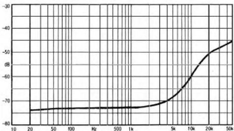
Disc input: stereo separation
