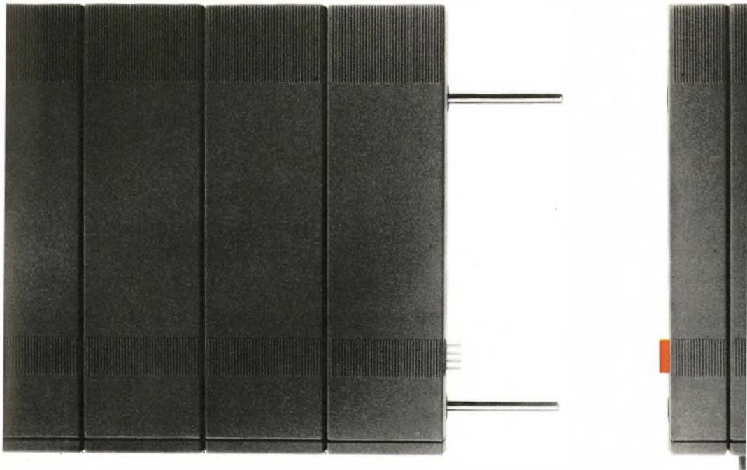
Between the power and pre-amp section can be plugged a series of modules to meet your specific needs. These modules are technically the very best and can extend to include up to 12 units selecting from FM tuner, headphone amplifier, tone controls, tape inputs, magnetic or moving coil cartridge and compact disc. As new technology is developed it will be incorporated into a module which you will be able to add to your system.
