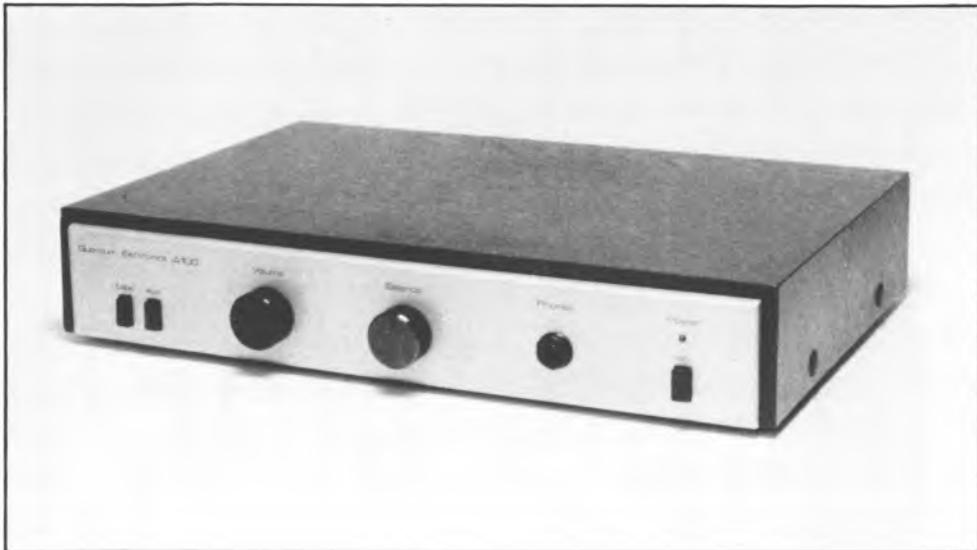
Quantum had been making the *IA-100* for some time, housing it in a plain black metal case, before updating the styling to a black ash wood-surround case with a silver grey front panel. In addition a moving-coil amplifier board may now be fitted internally at an extra cost of some £10.
