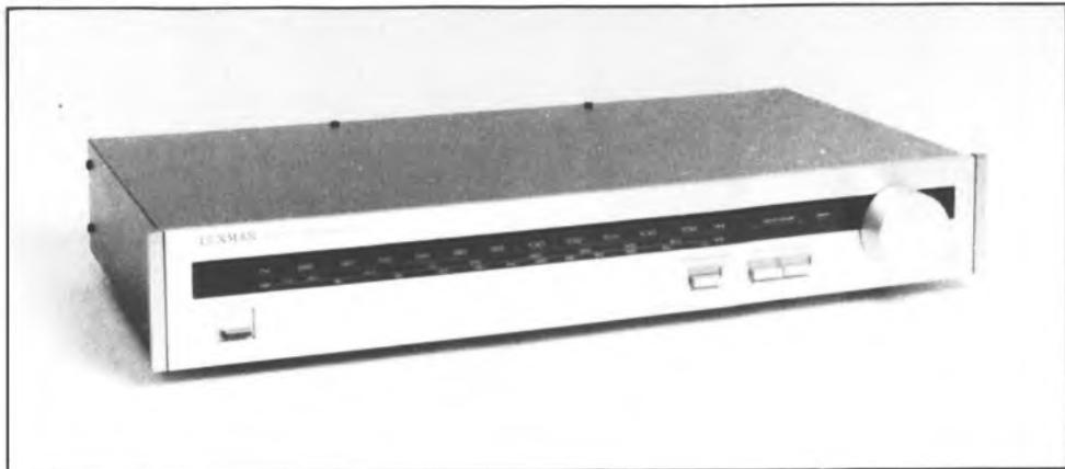
This is an 'old-fashioned' design in its use of a conventional FM front end with a normal tuning dial and a nicely weighted, free-spinning rotary control. The fast and convenient action of this system for seeking a wide range of stations must be set against the digital alternative, where manual tuning is more awkward but pre-set station selection is instant.
