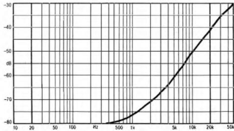
Disc input: stereo separation
