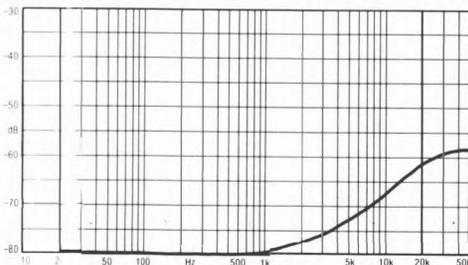
Disc input: stereo separation
