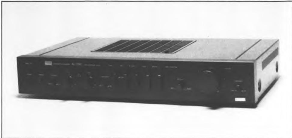
A budget model, the *101* is specified at 30W per channel and comes in a low, slim-profile satin black case. Tidily presented, the front panel offers a headphone socket, speaker muting, bass and treble controls, a high frequency filter, and selection of inputs: these are tape 1 and 2, aux/CD and tuner. A loudness contour switch is also provided and there are coloured lamps to show which input function is selected.
