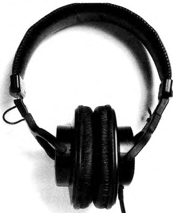
The *MDR-V6s* are larger than the other *V* models and have longer, oval circum-aural earpieces. These are set so that when the headband is at the top of the head the 'phones are at the right angle for one's ears, which seems to be a logical and effective system as these are reasonably comfortable headphones. However, for some ears they don't really fulfill the circum-aural precept of resting on the side of the head, being a little on the small side, and in my case resting partly on the ear.
