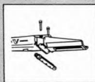
23mm diameter steel pillar, heat treated, ground and honed, carries two 17mm ABEC 7 ball races, widely spaced to resist tilt.
