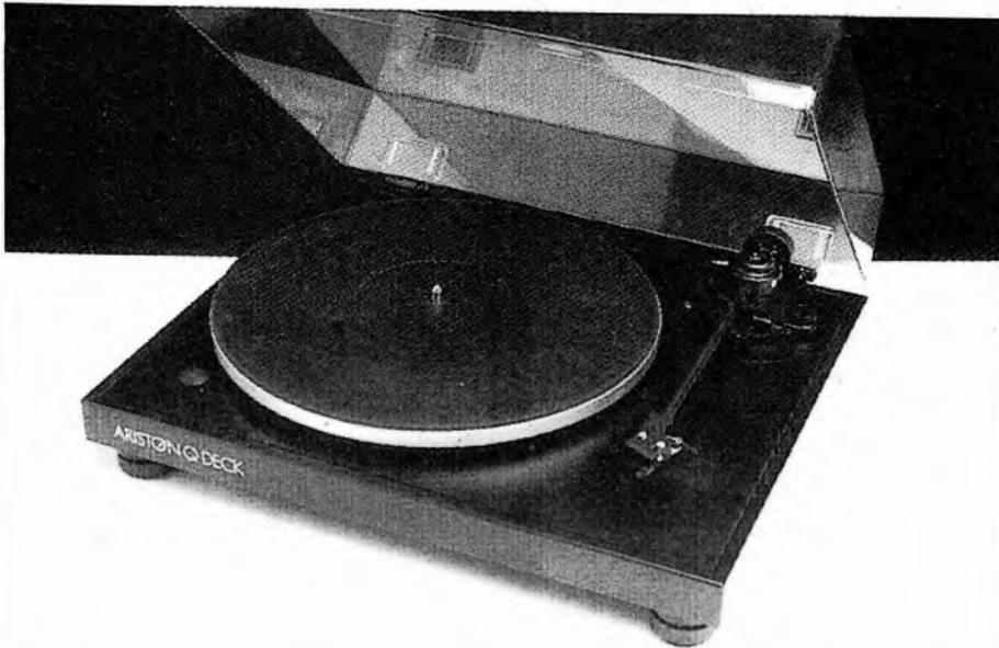
The *Q-Deck* is designed to meet the non-specialist user at least half way. The player works almost straight from the box. There's no suspension to adjust; the arm is non-interchangeable; and an Ortofon *OM10* cartridge is supplied fitted. Speed change is by a discreet dome switch, the motor being driven by a simple L-C oscillator.
