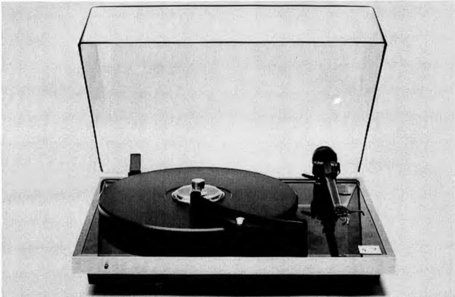
Townshend's new lower cost player retains the key Cranfield Institute of Technology derived features made familiar by the original *Rock*, including the radial silicone-filled trough which damps the arm/cartridge LF resonance by clamping the arm solid at low frequencies using an outrigger attached to the headshell. Various arms can be specified, but for this test the *Avalon* was fitted with a Rega *RB250*.
