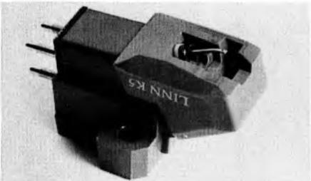
The *K5* is cheapest of Linn's K-series and appears to adopt the dual-magnet generator system used by Audio Technica in its cheaper MM cartridges. Indeed, both the elliptical stylus, crimped alloy cantilever and compliant damper are very similar to those employed in the *AT-420E*. Nevertheless, because of the *K5*'s lower bodyweight, its mean 14cu compliance makes it better suited to medium mass tonearms.
