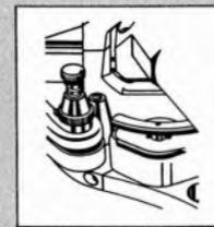
Understung weight housing corrects centre of gravity and provides non-reflective tone-arm termination. Adjustment leadcrew journalled in twin ball races with lever clamping.
