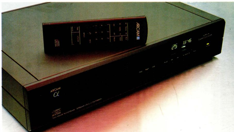
**K**een to keep the ball rolling in its favour, Arcam has just announced a series of mini-revisions to pep-up its long-standing *Alpha* CD player. Arcam has had the good taste to call the player *Alpha Plus* and not *Alpha SE* though certain of the mods, like sticking a rubber grommet over its 11.3MHz crystal, are pretty familiar.
