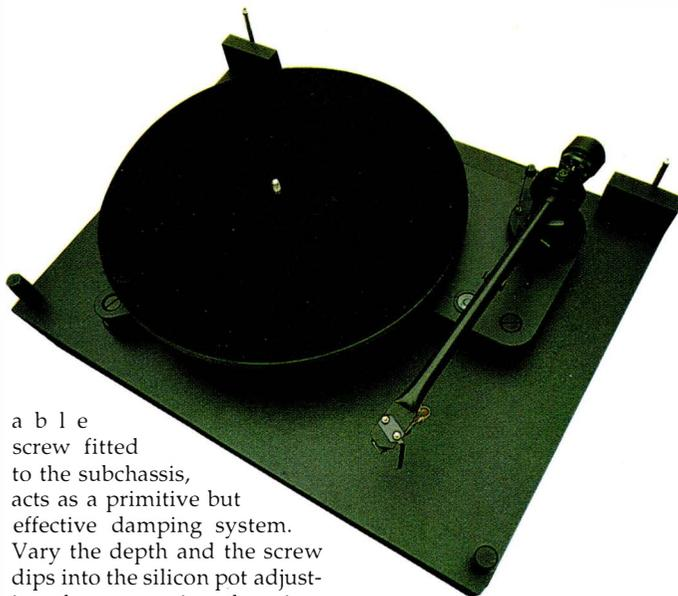
a b l e screw fitted to the subchassis, acts as a primitive but effective damping system. Vary the depth and the screw dips into the silicon pot adjusting the suspension damping. The combination of this damping and three adjustable cone feet makes the ensemble remarkably resistant to structure-borne feedback.
