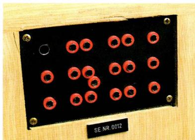
*This plate full of sockets is used to bridge a transformer which tailors the Agathon's response to your amplifier and listening room.*
