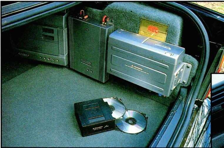
Power amps surround the *TS-W2RS* subwoofer while (right) the 12-disc CD changer partially obscures the *RS-P1* processor at the heart of the ODR system.
