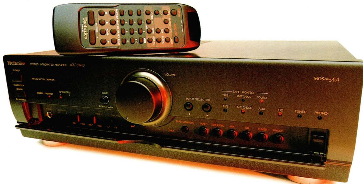
The £350 remote-equipped *SU-A800mkII* is a model of sophistication. It has logic-controlled input selection, local A/B speaker switching and motorised volume control; and there's even a cooling fan which is activated when the amp's pushed too hard (beyond 1A output). If the amp seems unusually heavy that's because it's built onto a shock-
