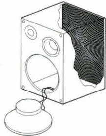
Place the flexible Deflex panel thru' the speaker cut-out and stick to the inside of the cabinet using the recommended adhesive
