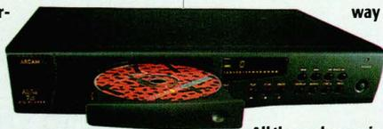
to 24 bits but, as I'm fond of repeating, this does not mean the player can or will offer a 24-bit (140-odd dB) dynamic range. In practice, the 7SE offers a 103.4dB S/N ratio and a practical dynamic range that's mid-way between that
