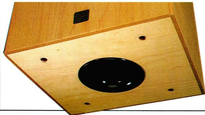
deep in order to accommodate a decent-sized main driver. The inside of the enclosure is used to excite two quite separate ports, differentially tuned to widen the operating band. The larger one fires down towards the plinth, with spacers to let the air in, while a much smaller port is up high on the rear panel. Bi-wire terminals are fitted on a substantial inset block fairly high up the back panel.
