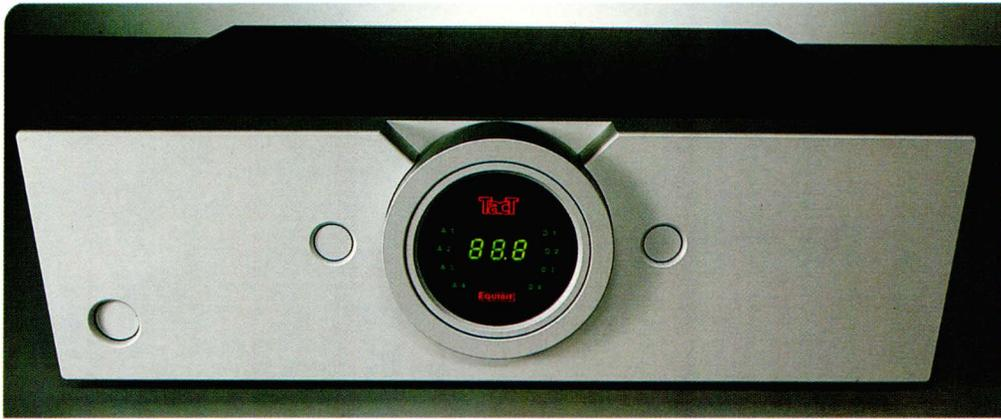
However, we mustn't confuse its immunity from *voltage* clipping with perfect tolerance of difficult loudspeaker loads. I squeezed some 160 Watts into 8 Ohm loads from the TACT, a figure that holds true under both continuous and dynamic conditions.
