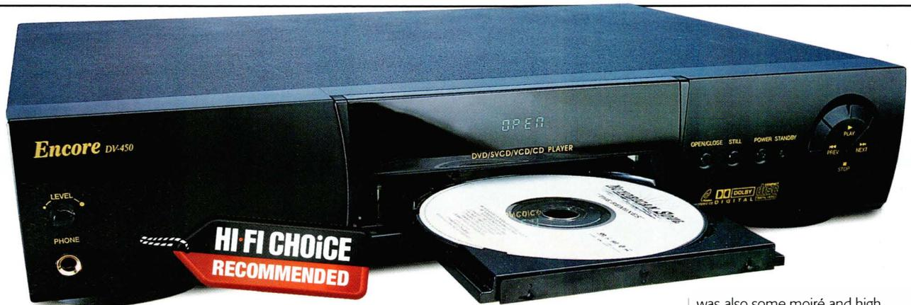
**A** Region 2 DVD player, the Encore has an on-board Dolby Digital decoder, and is easily hackable to work with Regional codes 1 through 6 via the remote control. As well as playing CD-Rs and RWs, the Encore will also play CDs which have been recorded with MP3 files, specifically 128kbps/44.1kHz files formatted to ISO9660. Dts datastreams can be reproduced through the audio digital outputs.
