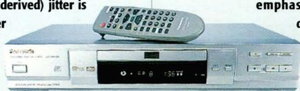
The player's ultrasonic spectrum is not unlike that of the Toshiba SD-100E, though there are in-band distortions seen here derived from digital processes within the player. The player will not respond to de-emphasis on CD-RW discs but normal silver CDs are flat to within +0.05/-0.15dB.
